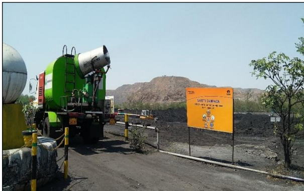
Water Mist Canon in coal stacking area
