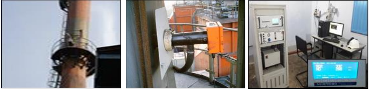
Continuous Emission Monitoring for Power House for PM, SO 2 & NO x data
