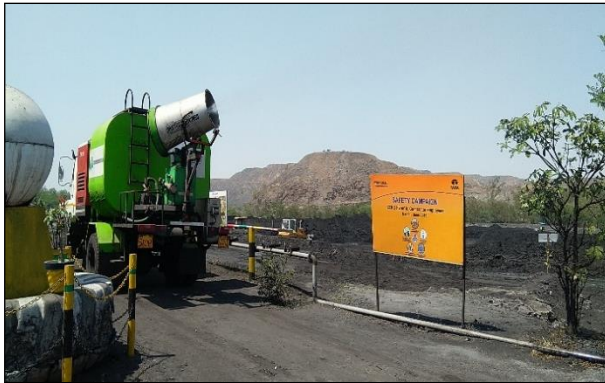
Water Mist Canon in coal stacking area
