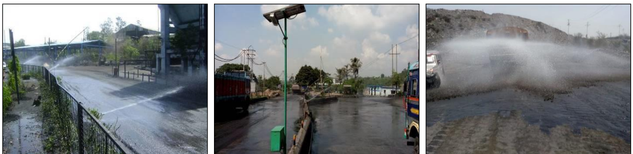
Use of fixed & mobile water sprinklers
