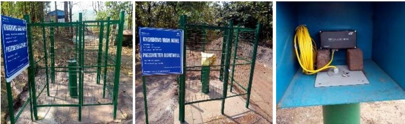
Piezometer (STP and Manganese) with digital recorder
