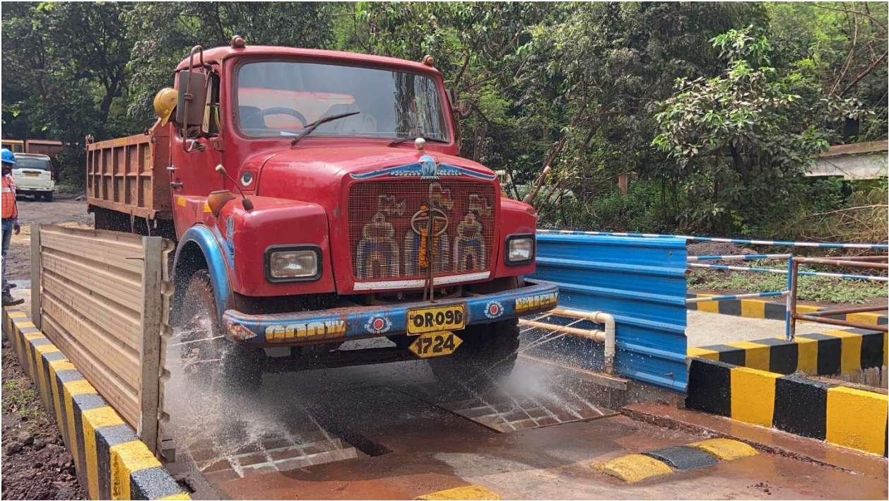
Fig.2 Wheel Wash System in Operation at Bamebari Iron & Mn Mine
