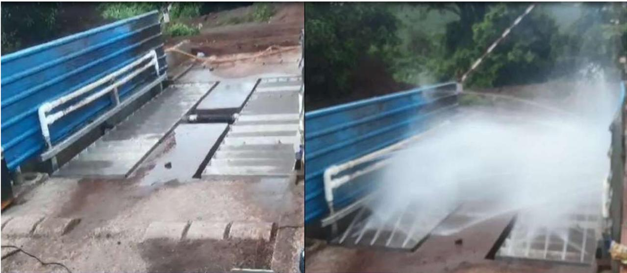
**Fig.2 Wheel Wash System in Operation at Joda West Iron & Mn Mine**
