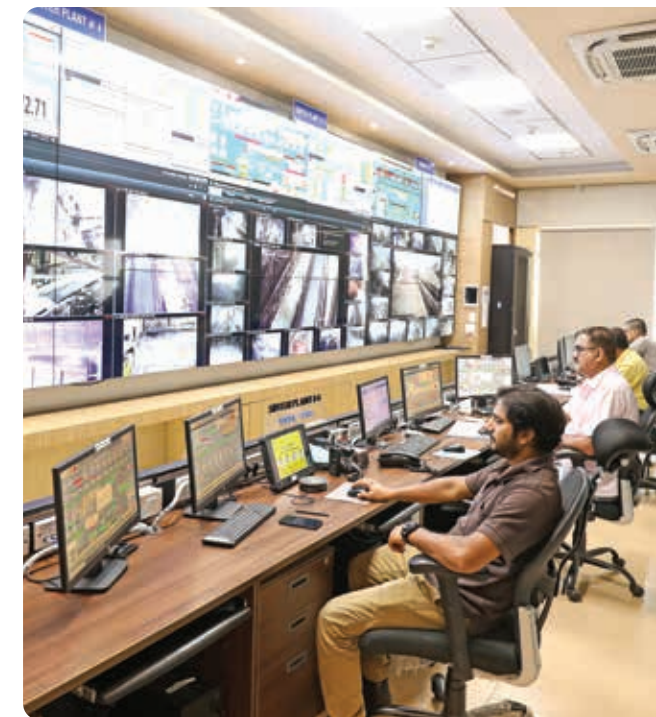
Integrated Sinter Plant Operations Centre (iSPOC) initiative to enable remote operations of Sinter Plant at Jamshedpur Works
