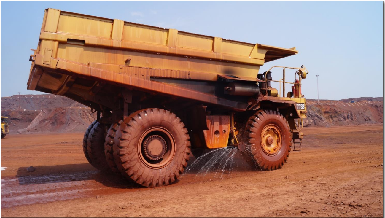
Mobile Water Sprinkling
