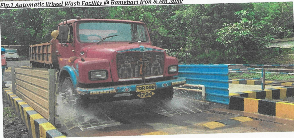
Fig.2 Wheel Wash System in Operation at Bamebari Iron & Mn Mine
