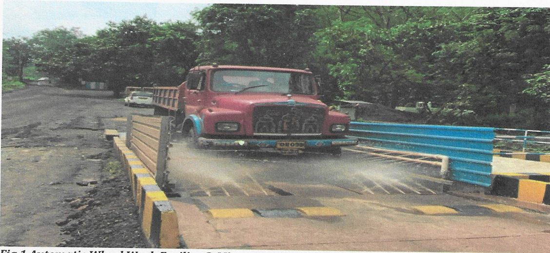
Fig.1 Automatic Wheel Wash Facility @ Mine Exit of Guruda Block of Tiringpahar
