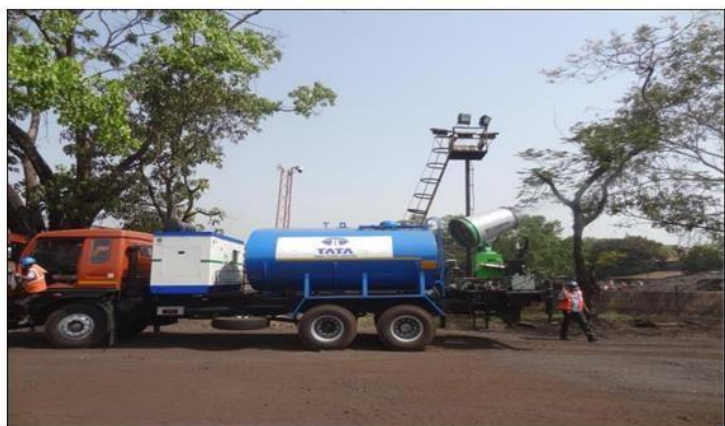
Mobile High Velocity Water Sprinkler cum Mist Canon
