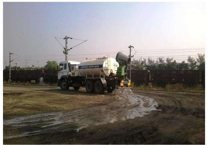
Water Sprinkling through truck mounted tanker
