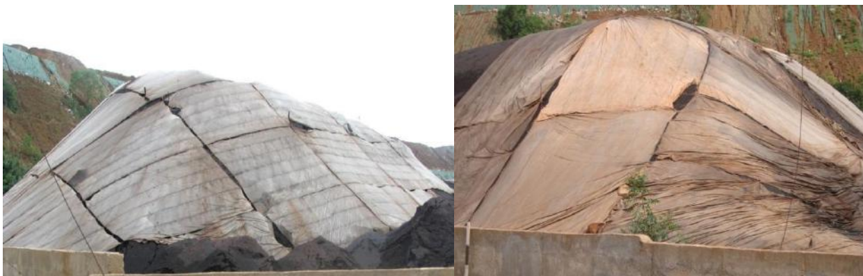
Concentrate Stack Covered With Tarpauline
