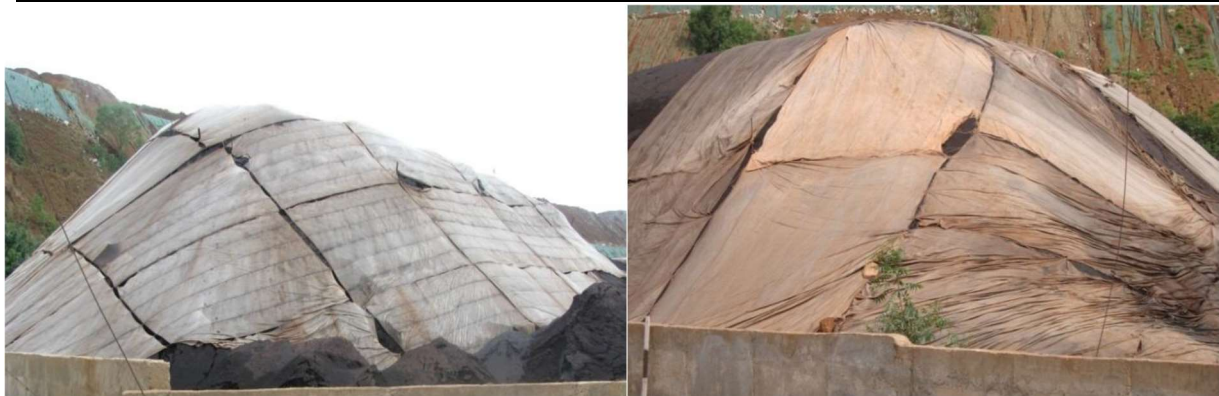
Concentrate Stack Covered with Tarpauline
